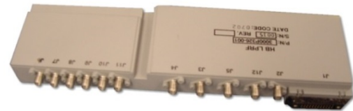
Fig 2: NW6418-28 6 to 18 GHz TWTA Exciter Amplifier
