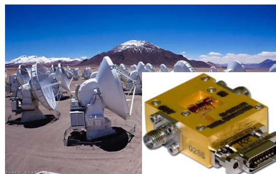
Figure 1: Cryogenic LNA Drop-In Module
