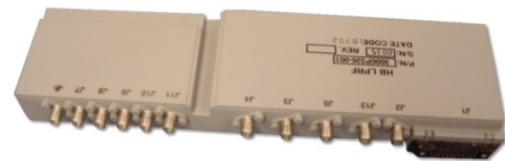
Fig 2: NW6418-28 6 to 18 GHz TWTA Exciter Amplifier
